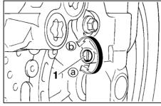
1. Compression damping force adjusting screw
